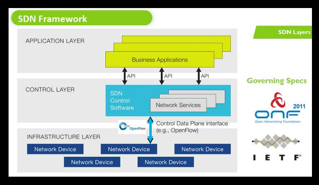
In SDN Architecture, OpenFlow protocol is key to entire topology. The group of few Intellects started working on OpenFlow specification in Stanford University & thereafter, in year 2011, The Open Networking Foundation also called as ONF was founded to promote SDN and OpenFlow. There are several workgroups created which started standardizing this OpenFlow protocol
