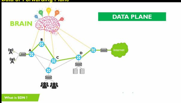
Let's First see how Data Plane works, in traditional network, there multiple switches & Routers having links connected to each other via line cards carry this traffic. This is where the data is actually moved from one device to another, as visible on-screen traffic is going all the way from Router A to Router B to Router C to Router D.
