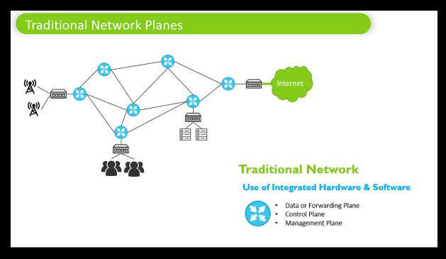
This is our traditional network where traffic is moving between various Switches & Router in order to reach its final destination
